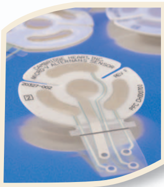
Proprietary multi-segment Micro-V Alternans™ Sensors minimize noise and artifact to permit data collection of alternans at the microvolt level.
